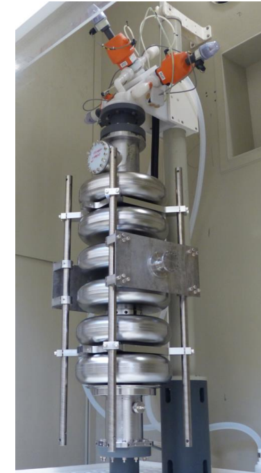
Treatment of ESS proto M-beta (2016): Standard 'BCP' Chemical polishing
