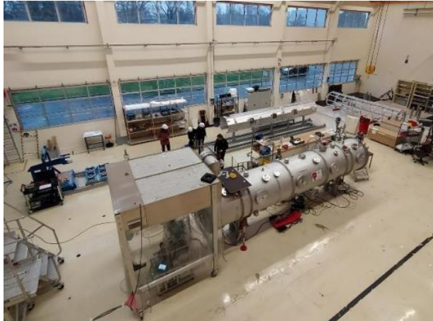
ESS Cryomodule assembly at CEA SACLAY On-going
