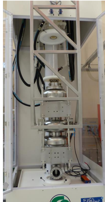
Treatment of \beta=1 SPL Cavity (2014) (EuCard): Electropolishing (EP)
