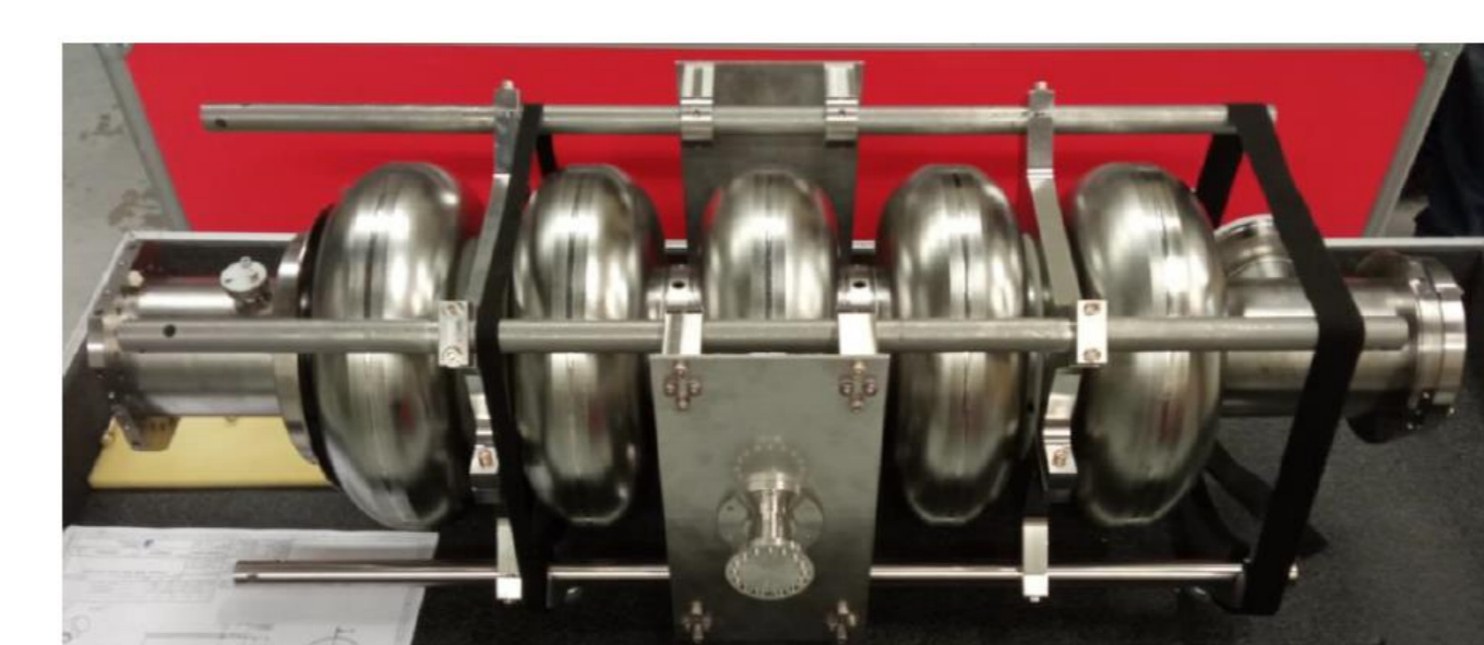
Eacc=52MV/m achieved after VEP followed by 2-step baking (75°C-120°C) (FERMILAB Recipe)
