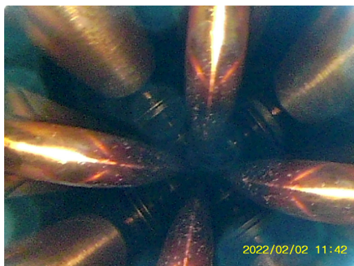
Figure 2: Condition of the RFQ vanes after RF conditioning and beam commissioning.
