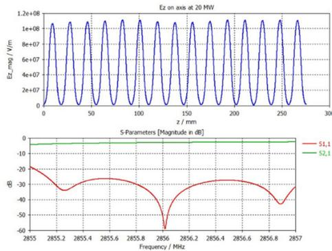
Figure 2. E-field profile along the axis (top) and S-parameters (bottom) for the new 15-cell NHS.
