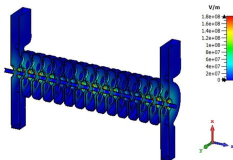
Figure 3. Surface electric field of the improved 15-cell NHS at 2856 MHz and 20 MW input power.
