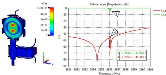
Figure 6. The electric field inside the SLED at 2856 MHz normalized to 5 MW input power (left) and its S-parameters (right).
