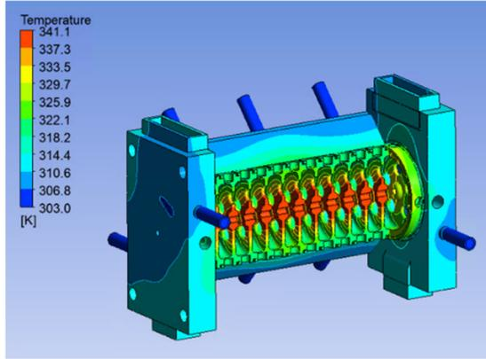
Figure 5. Steady state temperature field of the NHS with 0.117 kg/s water flow rate at 30°C.
