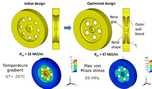
Figure 1: Initial and optimized cell design of the NHS (top). Thermal and stress maps for the optimized cell (bottom).
