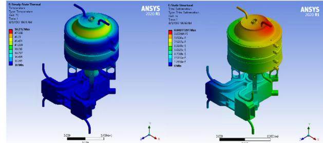
Figure 7. Thermo-mechanical analysis on the SLED.
