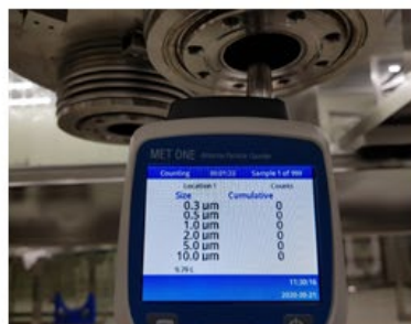
Particle count inside cavity "0"
