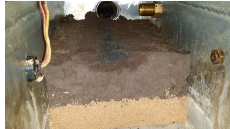
Decontamination cross section for a 10 MeV beam into a high-clay-content 5% contaminated soil
