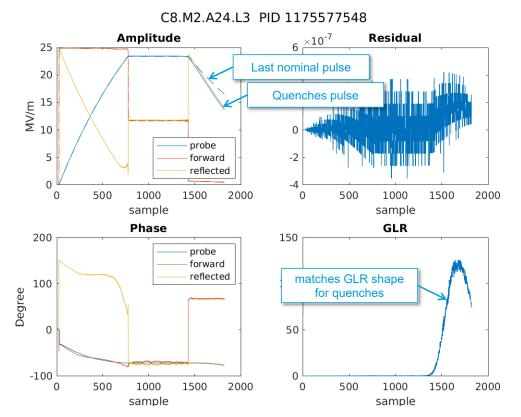
Algorithm accuracy  $a = \frac{TP + TN}{TP + TN + FP + FN}$  TP : true positive (accurately detected a quench) TN : true negative (accurately recognized a trip was not a quench) FP : false positive (a "fake" quench) FN : false negative (algorithm failed to identify a real quench)
