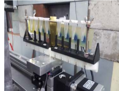
Wet plasmid samples in Eppendorf tubes. EBT-XD film placed behind samples, Manchester University (K. Small, R. Jones et al.)
