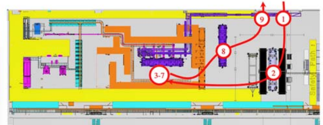
Figure 2. Flow of cryomodule testing phases in the different areas of the Test Stand 2
