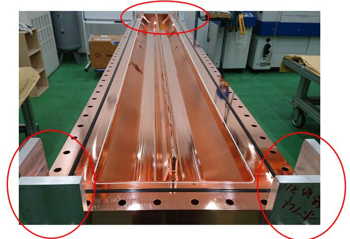
Assembled with a slide guide to avoid collision between vanes
