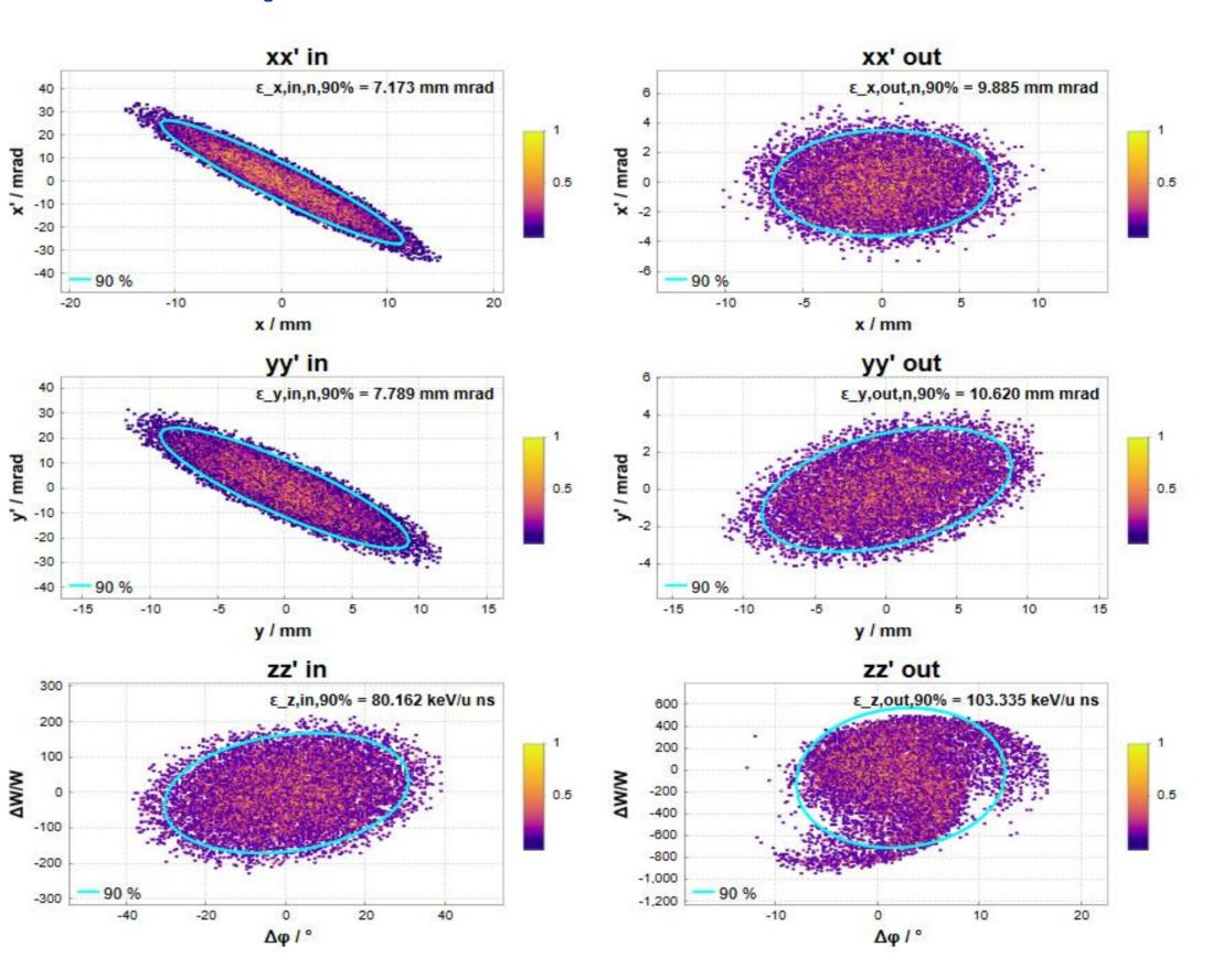
Simulated transverse and longitudinal input and output phase space portraits.
