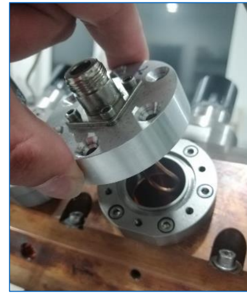
Fig. 5: Homemade Pick-up antenna
