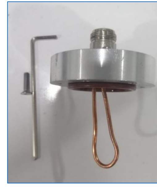
Fig. 5: Homemade Pick-up antenna
