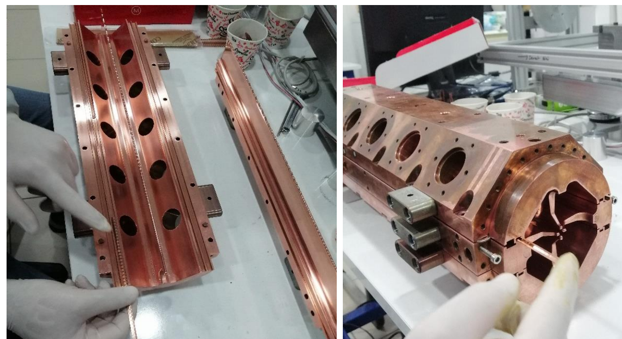
Fig. 8: Rf Fingers Placed in the Slots on the RFQ Test Module
