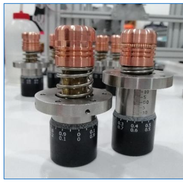
Fig. 4: Manufactured Tuners (10 Micrometer Precision)
