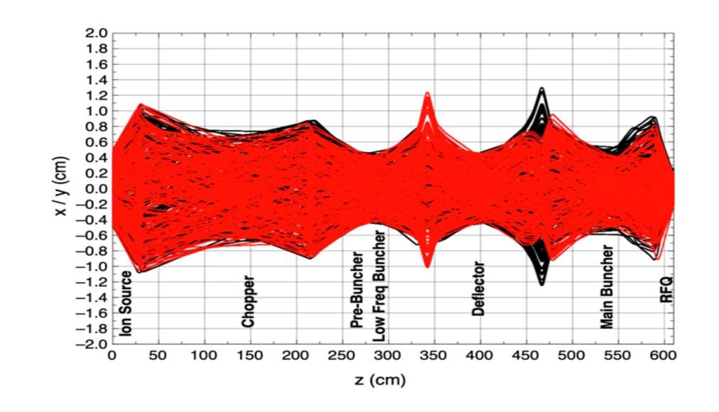
Particle trajectories in the injector beamline: (red) transverse, (black) vertical
