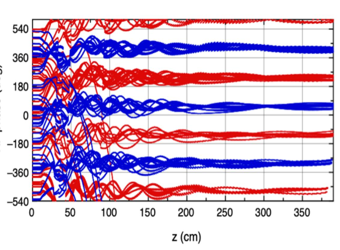
Phase trajectories in the two-component beam in RFQ: (red) H<sup>+</sup> beam, (blue) H<sup>-</sup> beam.
