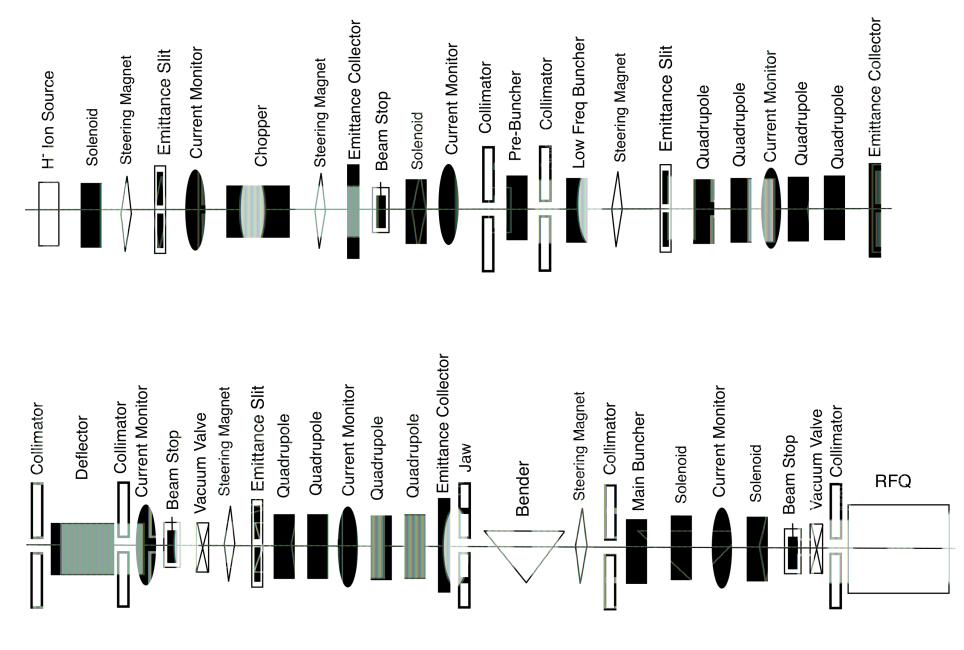
The layout of H<sup>-</sup> leg of the injector part with additional beamline elements.
