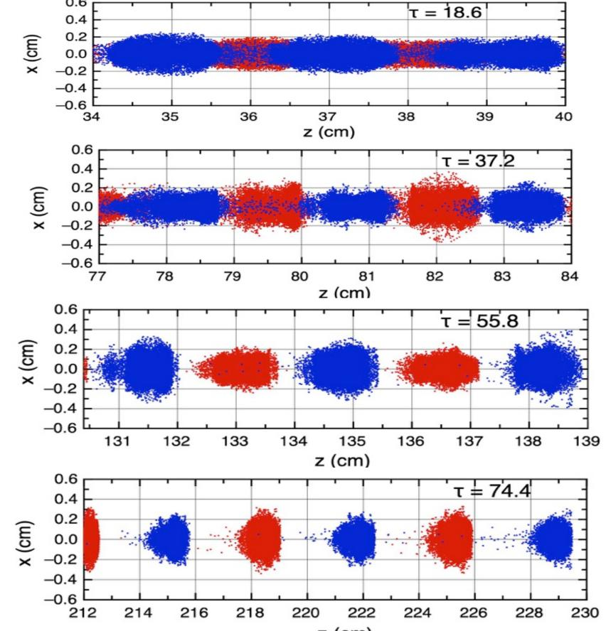
Formation of the two-component beam in RFQ: red) H<sup>+</sup> beam, (blue) H<sup>-</sup> beam. Numbers indicate RF periods.
