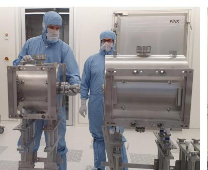
cleaning of cold BPM **Assembly of cold BPM** with ionized N<sub>2</sub> gun
