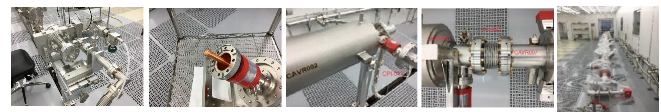
**Cavity String Assembly in the cleanroom**
