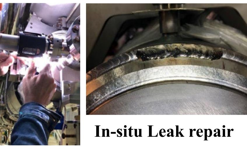
During the cold mass assembly at WS2 after the 2-phase circuit welding leak check, a helium vessel leak was found on an SRF cavity. This leak opened during cold test at the vertical test stand. The leak was repaired in situ. We revised the production workflow and introduced a new cavity jacket leak check step post vertical test.
