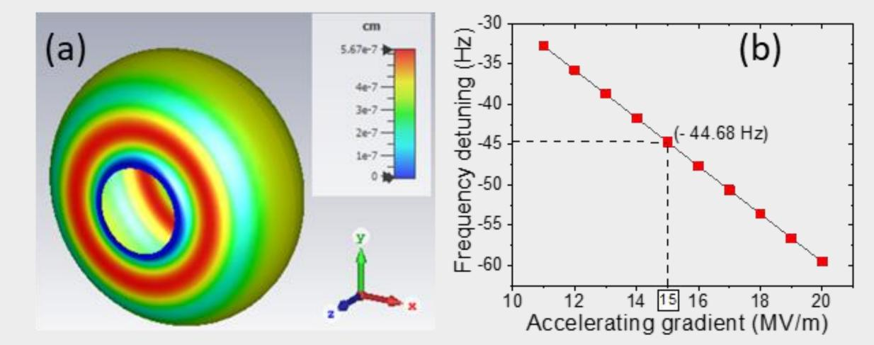
Fig.: (a) Displacement of the cavity after fixing the iris for  $E_{acc} = 15$  MV/m, (b) Resonant frequency detuning for different  $E_{acc}$
