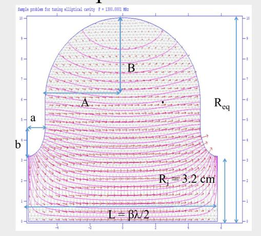
Fig.: Cavity design in 2D and geometry parameters
