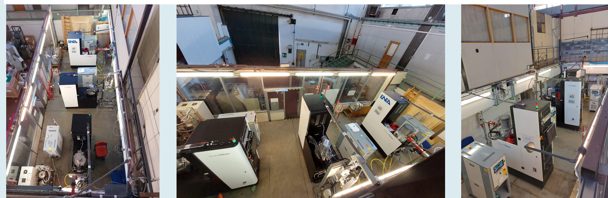
RF modulators area: (Scandinova K1) with Thales TH751A klystron and two Scandinova K100 with Canon E37325 klystrons.
