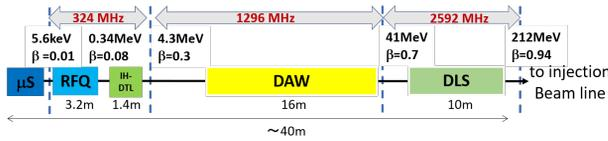
Figure 2: Configuration of the muon linac.
