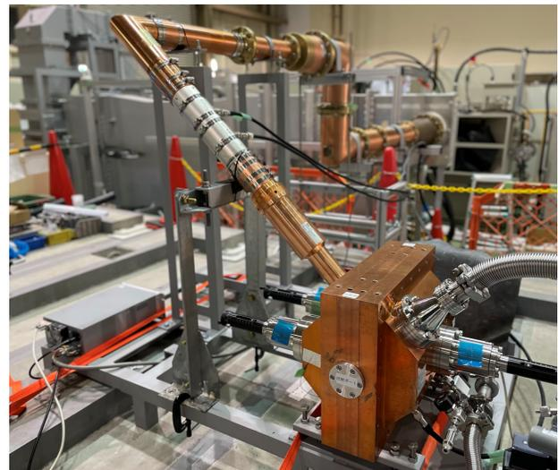
Figure 7: High-power test of the prototype IH.
