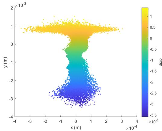
Figure 7: Simulated beam on the final screen, with TDC off and spectrometer magnet deflecting the beam by  $2.8^\circ$ , colour-coded according to the fractional energy offset  $\frac{dp}{p}$ .
