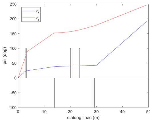
Figure 4: Horizontal  $\psi_x$  (blue) and vertical  $\psi_y$  (red) phase advance along the TDC beamline. The five black bars correspond to the locations of the five quadrupoles.
