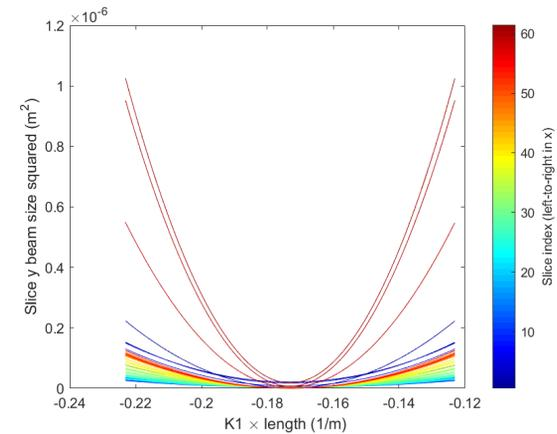
Figure 9: Quadratic fits to vertical beam size squared  $\sigma_y^2$  versus the product of quadrupole QH2's K1 value and length. Each parabola corresponds to a given beam slice as indicated in the colour bar.
