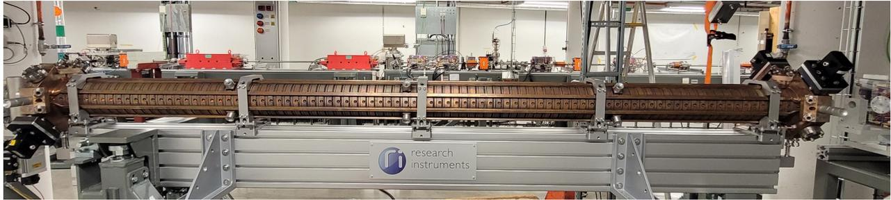
Figure 2: TDC structure installed in the beamline. The electron beam travels from left to right.
