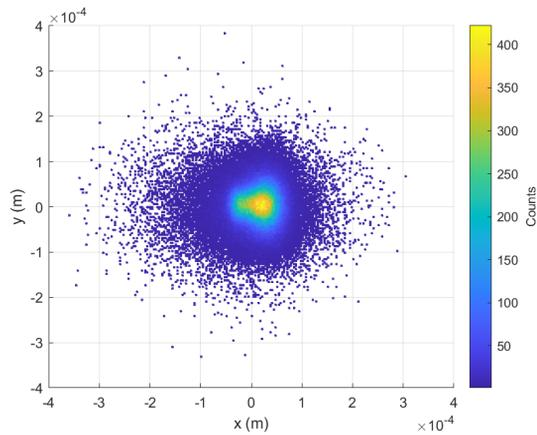
Figure 5: Simulated beam on the final screen, with both TDC and spectrometer magnet off, colour-coded according to beam intensity
