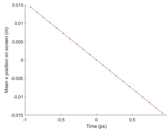
Figure 8: Simulated mean horizontal beam position on the final screen vs. beam arrival time at the TDC, relative to the RF zero-crossing, for an RF phase scan of  $\pm 1^\circ$ . The straight-line fit has a gradient of  $-0.0156$  m/ps.
