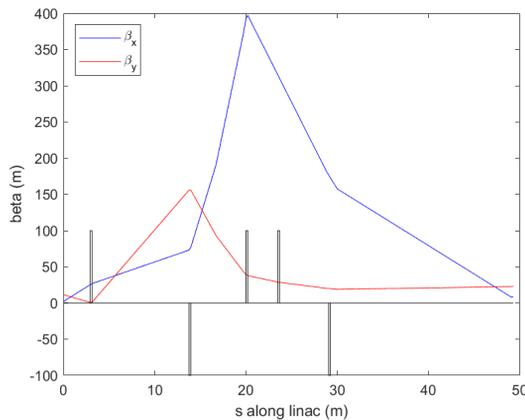
Figure 3: Horizontal  $\beta_x$  (blue) and vertical  $\beta_y$  (red) beta functions along the TDC beamline. The five black bars correspond to the locations of the five quadrupoles.
