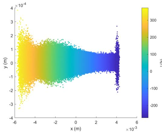
Figure 6: Simulated beam on the final screen, with TDC on and spectrometer magnet off, colour-coded according to beam arrival time  $t$ . Negative time corresponds to the head of the bunch.
