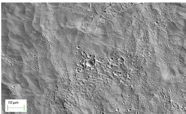
Figure 6: SEM imaging showing the breakdowns triggered by the LES experiment, on the Nb irradiated cathode, using secondary electron detector.
