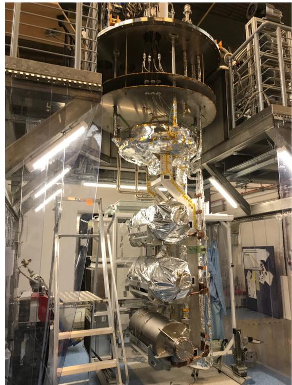
Figure 1: Photograph of CSI on stand with three jacketed cavities installed (top and middle cavities dressed in MLI jackets)
