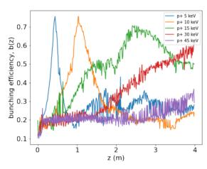
Figure 5: Bunching efficiency as a function of distance from the buncher center, for ESS-Bilbao proton beam with different extraction voltages.
