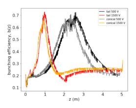
Figure 3: Bunching efficiency as a function of z for different geometries and electrode voltage, for HIE-ISOLDE beam.
