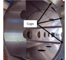
Figure 5: Gaps in between the skeleton and the vacuum vessel.
