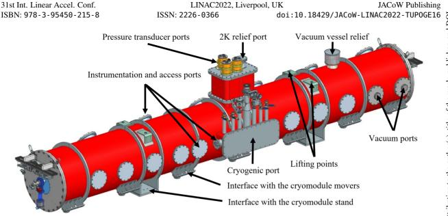
Figure 4: Standardized interfaces on the SSR and 650 cryomodules.
