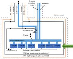
Figure 3: Schematic of the cryogenic lines.
