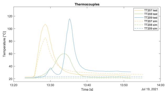
Figure 5: Measured (solid) and Simulated (dotted) temperature evolution after a multipacting event occurred.
