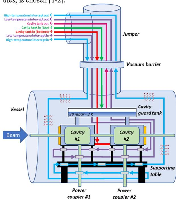
Figure 1: The simplified flow schematics of the MINERVA prototype SPOKE cryomodule.
