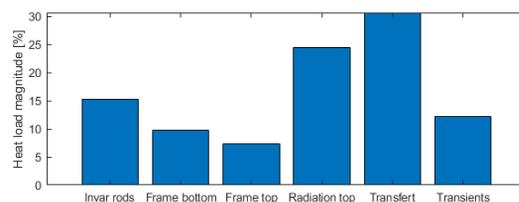
Figure 3: Instantaneous heat load distribution on the 2K tanks, at the same condition as the measurement.
