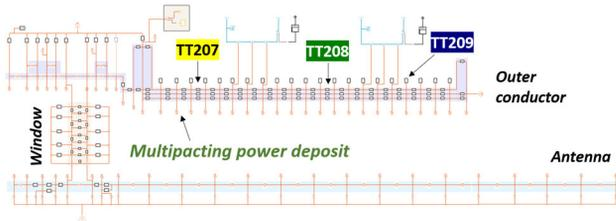
Figure 4: Simscape model of the MINERVA coupler.
