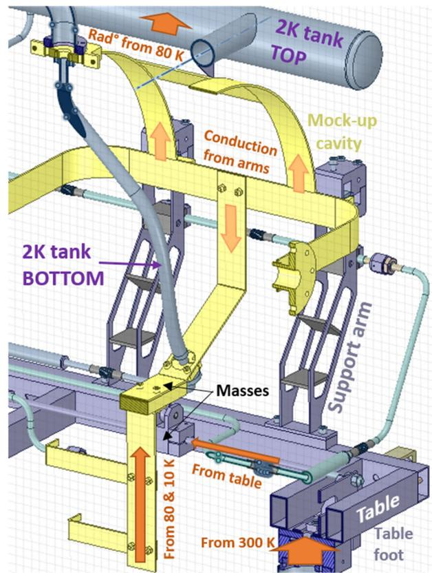
Figure 2: Cross-section of the MINERVA prototype cavity string supporting system, and main heat fluxes.
