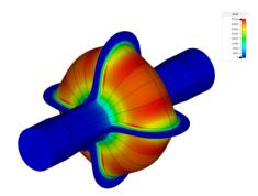
Figure 4: Magnetic field in the 1.3 GHz SWELL cavity for 1 Joule of stored energy.
