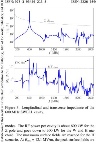
Figure 3: Longitudinal and transverse impedance of the 600 MHz SWELL cavity.
