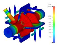
Figure 2: Electrical field at the H working point of the FM on the SWELL cavity surface equipped with one FPC and two RF plungers (not visible on the picture). The field scale is cut to 20 kV/m for easier understanding of the field distortion in the slots.
