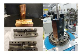
Figure 8: 6 GHz split cavities after machining and surface coating.
