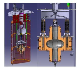
Figure 7: V5 vertical cryostat equipped with the 1.3 GHz SWELL cavity.
