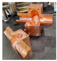
Figure 6: First 1.3 GHz SWELL cavity machined.
