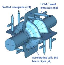
Figure 1: SWELL 2-cell 600 MHz cavity RF volume.
