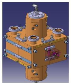
Figure 5: 3D view of the mechanical design of the 1.3 GHz SWELL cavity.
