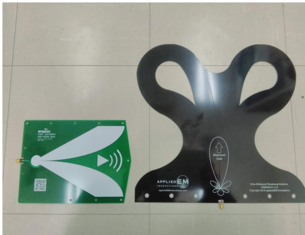
Figure 5: The ultra-wideband antennas for detecting signals from the interactions with plasmas.
