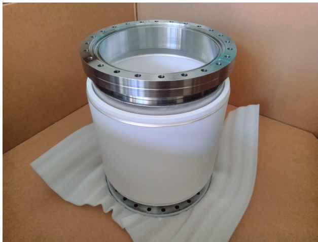
Figure 4: The plasma chamber made of ceramic for the outside detection of radiation signals.
