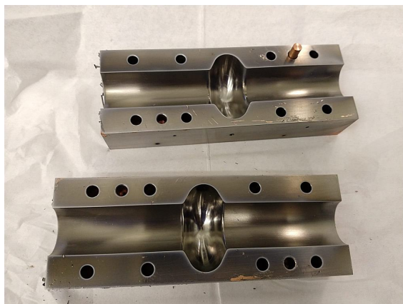
Figure 2: Cavity A coated with niobium.
