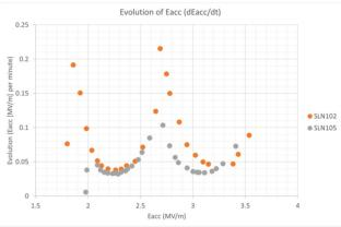
Figure 4: Evolution of Eacc in time for two LB cavities: SLN102 and SLN105.
