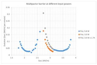
Figure 5: Evolution of the MP barrier for SLN111 with 2 different injected powers.
