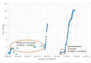
Figure 7: Multipactor barriers for cavity SLN122. The small barrier at 0.4 MV/m is visible.
