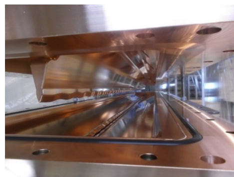
Figure 2: In process of assembling three-layer structure RFQ.
