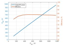
Figure 7: Measured output RF power and efficiency vs. DC power for the 1 kW module.
