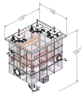
Figure 5: Engineering design of the RF sweeper with overall dimensions in millimeters (in brackets) and inches.
