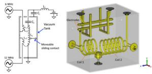
Figure 2: Schematics of dual frequency RF sweeper (left) and its 3D model (right).
