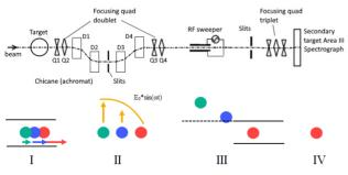
Figure 1: Layout of the ATLAS in-flight RIB facility (top) and the scheme of rare isotope RF separation (bottom).
