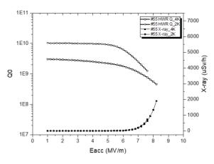
Figure 3: Quality factor and x-ray radiation of No.55 HWR: the square line and circle line represent 4K and 2K data, respectively.
