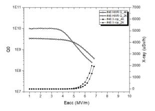
Figure 2: Quality factor and x-ray radiation of No.46 HWR: the square line and circle line represent 4K and 2K data, respectively.
