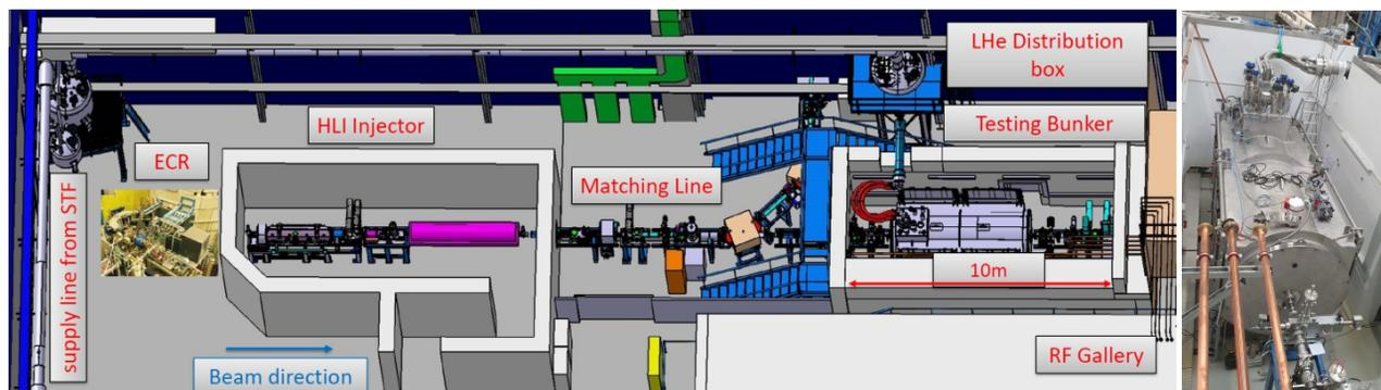
Figure 2: 3d Model of the testing area at GSI (left) and photograph of cryostat installed in testing area.
