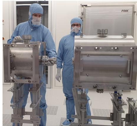
Figure 6: Integration of rf-power coupler into CH2 cavity (top panel) and interconnecting the CH2 and S2 with bellows (bottom panel) in clean room CR2 .
