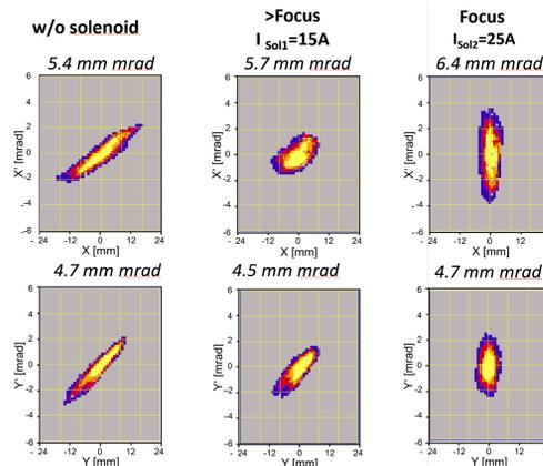
Figure 4: Transverse beam emittance.
