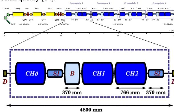
Figure 1: Layout of the HELIAC (top) and of the first cryogenic module i.e. "Advanced Demonstrator" (bottom).
