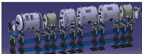
Figure 5: 3d Model of cold string assembly in clean room.
