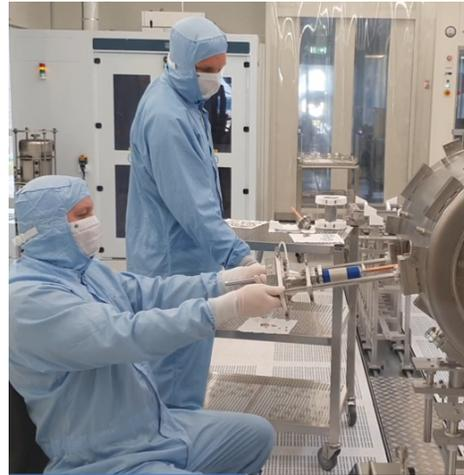
assembly of S2 and CH2 with bellow
