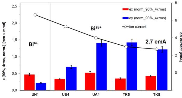
Figure 5: Transversal  $\text{Bi}^{4+}/28+$  emittance along UNILAC [17].
