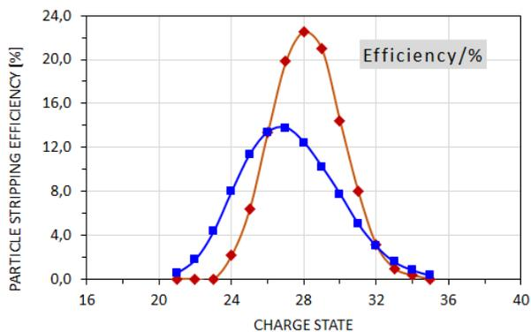
Figure 2: Uranium beam stripping efficiency for two different stripper targets ( $N_2$ (blue) and  $H_2$ (red)).
