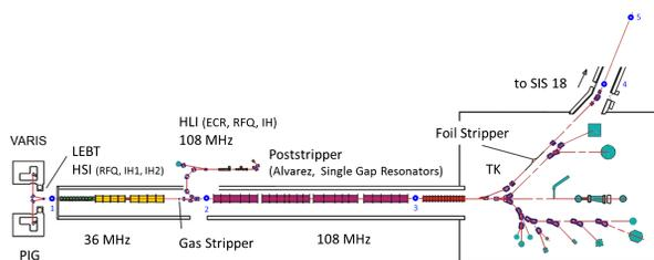
Figure 1: Overview of the GSI Universal Linear Accelerator (UNILAC) [1]; numbered blue dots mark positions of installed emittance measurement devices.
