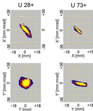
Figure 7: Transversal emittance at TK8, applying pulsed hydrogen gas stripping for 4.0 eMA of  $\text{U}^{28+}$ , 1.0 eMA of  $\text{U}^{73+}$  (2022).
