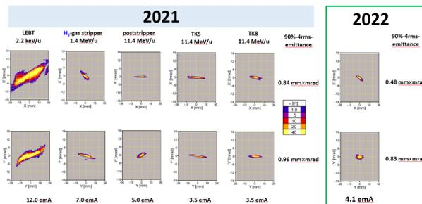
Figure 4: Transversal  $U^{4+}/28+$  emittance measurements along UNILAC.
