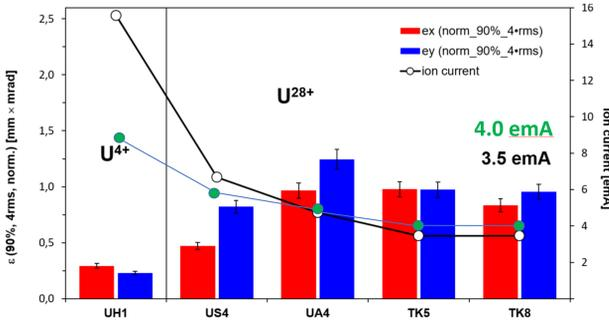
Figure 6: Measured transversal  $\text{U}^{4+}/28+$  emittance along UNILAC for the 2022 and 2021 campaign.
