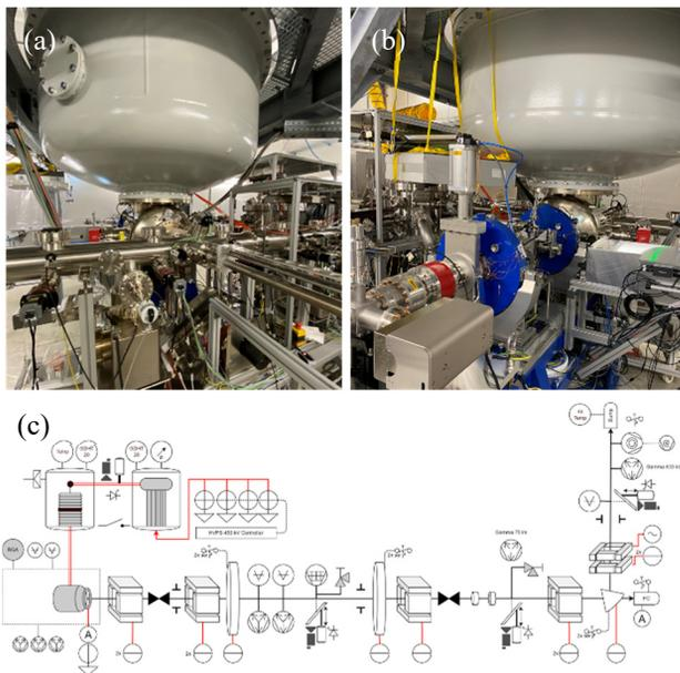
Figure 3: (a) Photograph of the BTF from behind the gun, also showing a part of the photocathode production and transfer system, (b) photograph of the BTF from the beam-line side with two solenoid magnets and beam current monitors, (c) schematic overview of the BTF and its components.
