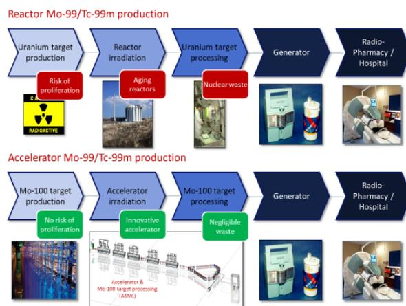
Figure 1: Innovative production of Mo-99 from accelerator irradiation compared to traditional production in a nuclear reactor from Uranium targets. Courtesy of IRE.
