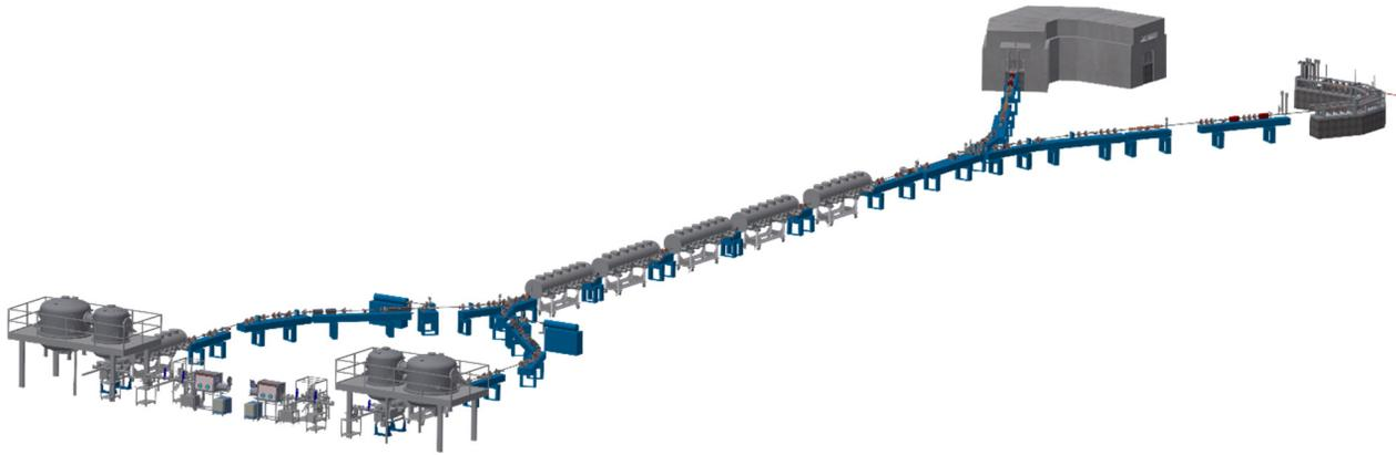
Figure 2: 3D Model of the LightHouse accelerator. Two parallel injectors (left) will increase the availability of the system. The electron beam will be split at 75 MeV into two arcs to illuminate the target (top right, details not shown) from both sides simultaneously. The last part of the beamline will be designed to tolerate the high radiation background from the target. The shielding is only shown for the left arc but would be applied for both sides.
