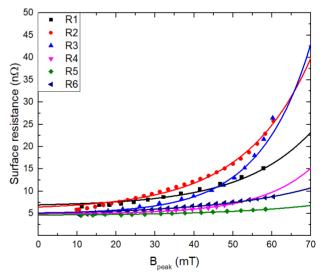
Figure 4: Magnetic heating effect of the surface resistances for the QWR cavities.
