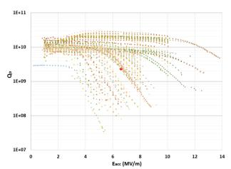
Figure 2: Q slope measurement for the HWR cavities at 2 K.
