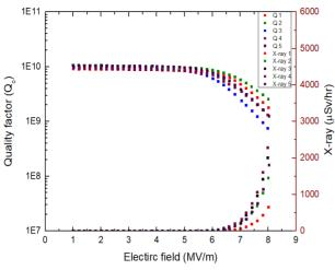
Figure 5: Quality factor vs accelerating field for the HWR cavities [14].
