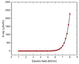
Figure 6: X-ray vs accelerating field for the half-wave resonators (HWRs) [14].
