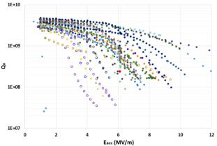
Figure 1: Q slope measurement for the QWR cavities at 4.2 K. This data shows the failed and passed QWRs. The number of the QWRs is 22 and all of them are passed.
