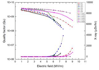
Figure 3: Q slope measurement for the QWR cavities.
