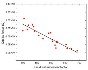
Figure 7: Quality factor vs x-ray field enhancement factor for the half-wave resonators (HWRs) [14].
