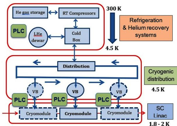
Figure 1: SC Linac, main cryogenic components.
