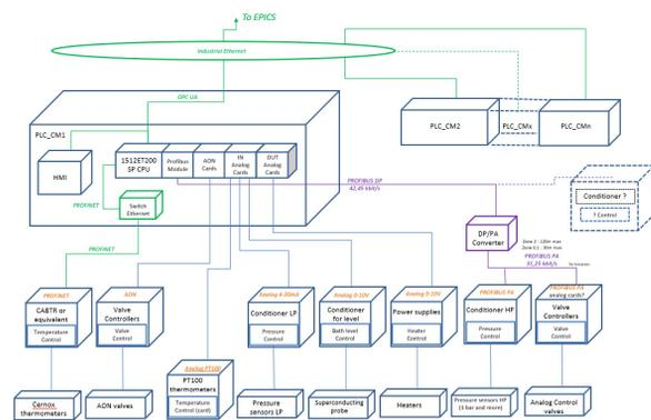
Figure 4: Generic system architecture for the cryogenic control system at field level.
