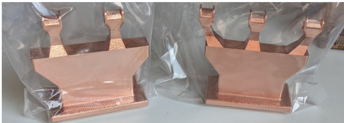
Figure 5: First iteration of AM stainless-steel IH-structures after polishing and galvanic copper-plating.
