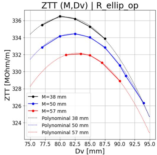
Figure 3:  $ZTT$  analysis for the values  $M = 38, 50, 57$  mm as a function of  $Dv$  and maximising the value of  $R_{ellipse}$ .
