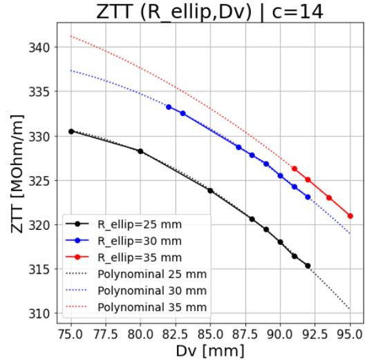
Figure 2:  $ZTT$  analysis for  $R_{ellipse} = 25, 30, 35$  mm as a function of  $Dv$  in the flat-walled cavity.
