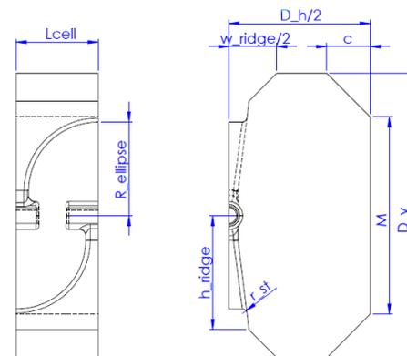
Figure 1: Front view (right) and lateral cross section (left) of half standard IH cell.
